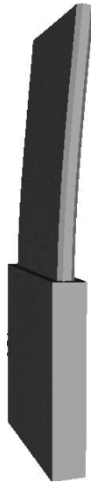
Figure 43 – Deformations inferred by MAMGN for Mode 1.
