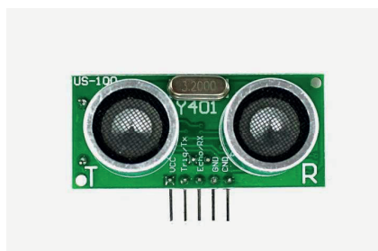
Figura 2: Sensor Ultrassônico (US-100). Fonte: QuartzComponents. Disponível em: https://quartzcomponents.com/collections/distance-sensor/products/us-100-ultrasonic-sensor-distance-measuring-module-with-temperature-compensation
