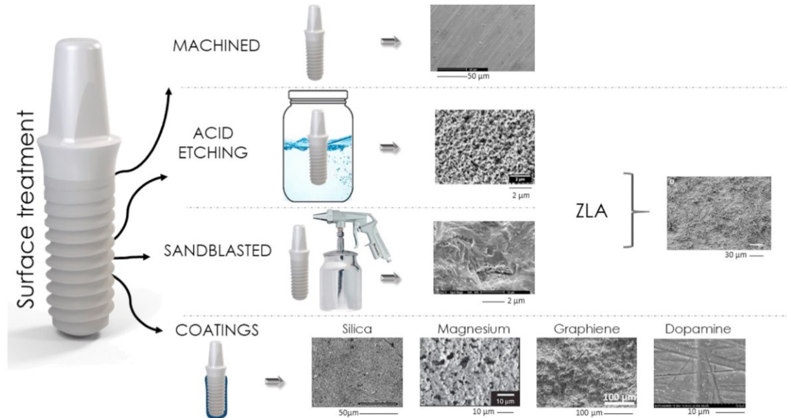
Figure 1 - Schematics and SEM images on different zirconia surface modifications: machined (LIU et al. , 2015), acid etched (QUENTINFLAMANTA et al. , 2016), grit blasted (LIU et al. , 2015), ZLA (ROEHLING et al. , 2017), and multi-layered coatings (KAROLINE PARDUN et al. , 2015; LARANJEIRA et al. , 2014; LIU et al. , 2015).
